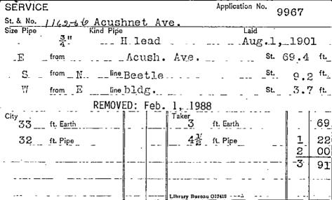
10/27.87-Renewed from ½' outside curb stop to a point 3 ft. 3½'-3/4" copper tubing, 3/4" curb stop, Caldwell stop box, 2-3/4x3/4 lead to cop. adapt. (xxs & xs). 2/1/88-Serv. shut off at tap & abandoned in ground.
