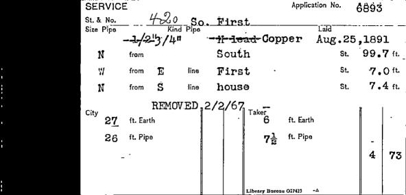
8-28-51, ser leak, replaced old lead pipe from tap to cellar inside using 32 ft. 3/4" copper tubing type K, soft. Bill No. 47069. Tap reamed. 5/8" tap at main. Pipe formerly went through manhole. Now pipe laid around the northside of the manhole. 2/2/67, shut off at the corp. tap; coupling was removed and returned to repair shop; stop box & pipe abandoned in ground.
