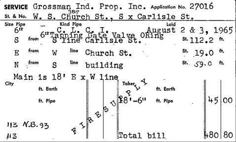
1-22-94 The 6" fire supply gate valve was shut off& gate box remove Cut the 6" line at a point 5ft. W x tapping gate valve & installed a 6." mech. plug. E x W line church st. 14ft st. cut 9' x 4' Warrenite
