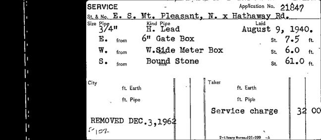
Service removed - Dec. 3, 1963 - was completely removed, shut off at tap, connection cut off, lead pipe and stop box were removed. Now supplied by Ser. #26228.
