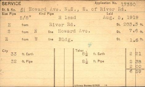
5-7-93 Canessa Const. cut off the 6" main & removed aling with this service. All material removed. This service was found cut off at tap-date unknown 5-7-93 Canessa Const. cut off the 6" main & removed along with this service. All material removed. This seervice was foundcut off at tap-date unknown.
