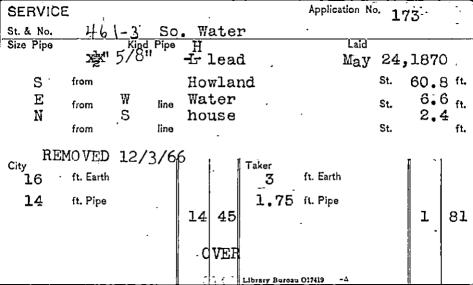
Replaced 2" L. Lead with 5/8" H. Lead, Using 16' pipe 4.48 -----16 - 5/8H. Lead 1 5/8 Stop 5-2-39 1# Solder 12/3/66, shut off at corp tap & coupling & stop box (complete) were removed-and-returned to the repair shop. Pipe was abandoned in ground.
