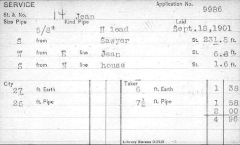
Sept. 9,1953, ser. leak, renewed from main to 1 ft. from main using 1 ft. 3/4" cop.tubing Tap reamed. 1 wiped joint.
