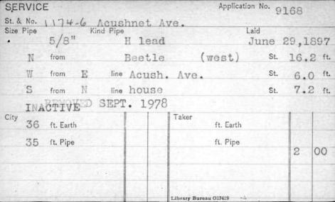
2/2/67, renewed from 1 ft. outside curb stop to 2 ft. inside curb stop; 3 ft. 3/4" copper tubing used; 1 3/4" curb stop.
