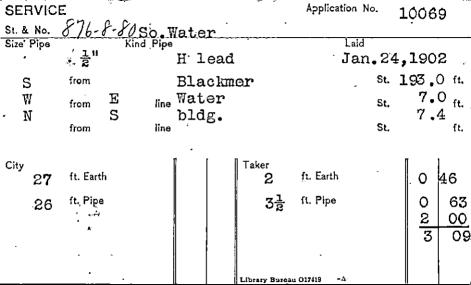
Sept. 9,1953, ser. leak, renewed from curb stop to inside. Tap reamed. Used 12% of 3/4" cop. tubing type k. I wiped joint. Bill No. 47863.
