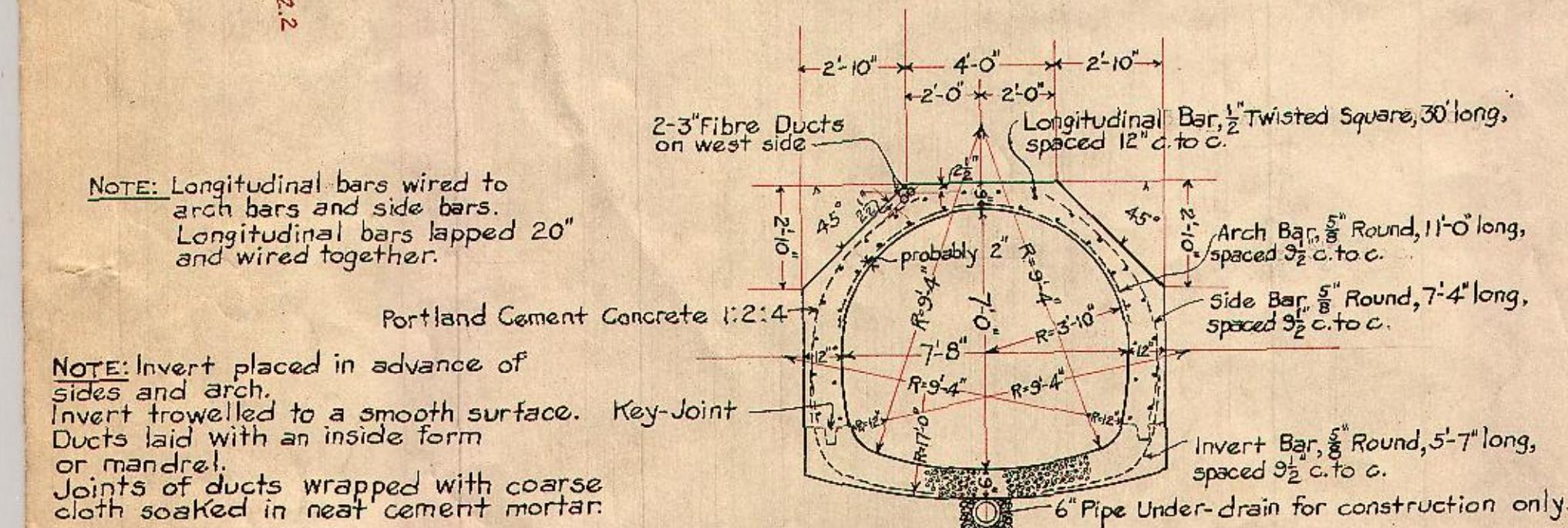
**SECTION OF 7'-0"X7'-8" REINFORCED CONCRETE SEWER
