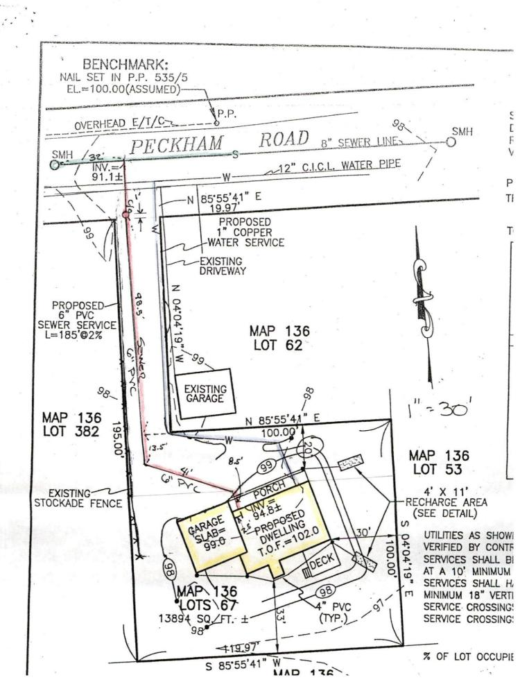
Lot of PECKHAM ROD. OVERHEAD E/T/C- -- 8 PECKHAM ROAD 8" SEWER LINE SMH 32' INV.= 91.1± 12" C.I.C.L. WATER PIPE -N 85'55'41" E 19.97' PROPOSED 1" COPPER -WATER SERVICE 1=40 -EXISTING DRIVEWAY PROPOSED—6" PVC
