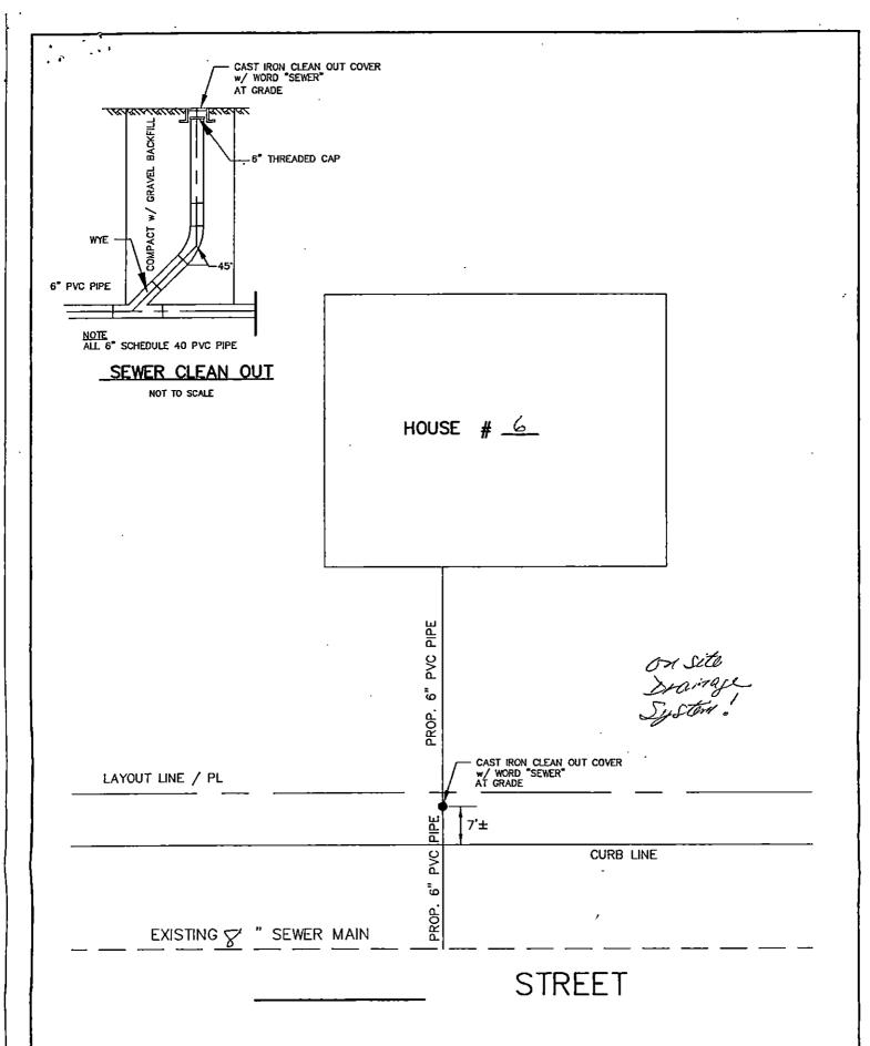
PROPOSED SEWER STUB DIAGRAM
