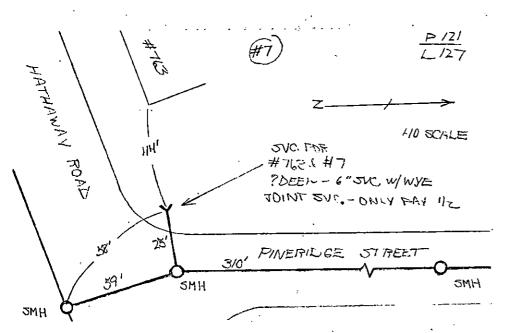
ACREEMENT ON FILE-YAWAHTAH 50 HAVE A JOINT SEWER 2934WD - 8572 04 151-1 100 AND TIE BY FORCE MAIN BOTH HOUSES TO ONE PULL GONTRACTOR TO HOOK UP JUNOULA . WOLL OF 3AA CLAM SOROT SIL STUB. COUNTECTIONS AT HOUSES CARATTY SEWER TO EVISTOL A WUS TOW CHUDD : 510H SEL9-266-805 THANGHER CIST - FOLDASINOD 78255 TMR3 TT 3687 3WG 7 75 38385 THASE OX YAWAHTAN 837 # YACEDHI 30-20-1 FRIM 400
