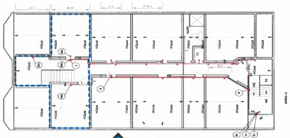
3RD FLOOR SPRINKLER PLAN
