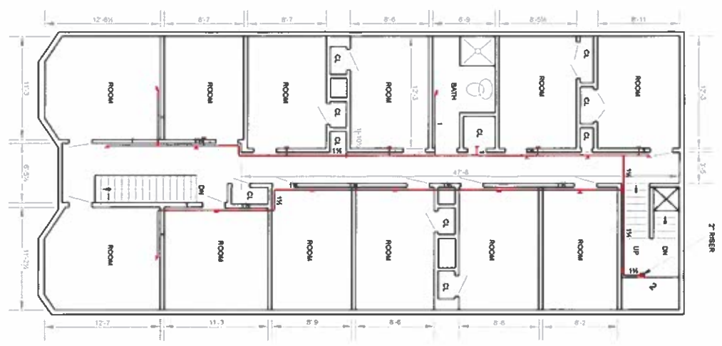
2ND FLOOR SPRINKLER PLAN
