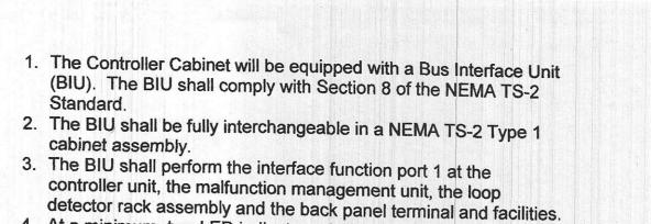
4. At a minimum, two LED indicators shall be provided on the BIU front panel. One indicator shall serve a dual use; as a power on indication and as a diagnostic indicator for proper operation of the device. The second indicator shall serve as a transmit indicator illuminating each time data is transmitted.
